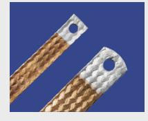
• Braided Flexible Busbars are made of electrolytic copper (bare or tinned) wires and afterwards braided wires are fixed with pressed (without annealing) Cu-ETP Pipes at the ends. These Pipes (Connection surfaces) can be tin or silver plated if requested. Holes can be punched at these ends according to your requirements
