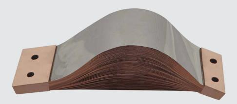
They are manufactured by combining Cu-ETP strips with a thickness between -0,10 mm and 0,20 mm to provide the desired properties and riveted under a press. Contact surfaces are additionally reinforced with thicker plates. - These bars are manufactured according to customer requests and drawings.
